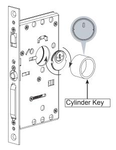
Note: Notches on cylinder must be parallel with the horizontal plane when fully screwed into lock body.
